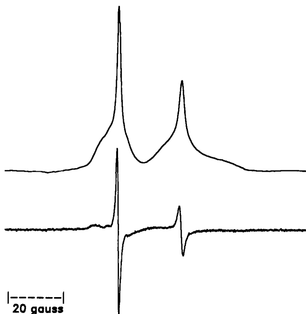
Fig. 4. The first derivative and adsorption spectra of d_8 ^{15}\text{N} 17-DSA labeled porcine stratum corneum. Note how the immobilized signal dominates the integrated spectrum.
